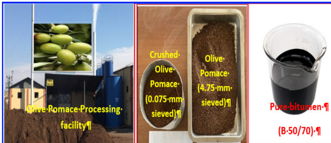
Figure 1. PO facility and crushed sieved PO sample
